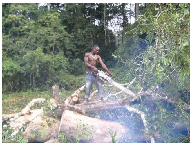
Power saw operation at Kasewe Sawmill cutting a Anisophyllea laurina tree, used mostly as construction poles.
